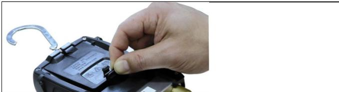
1. Fold out the suspension device, loosen the clip and remove the cover of the battery compartment.
